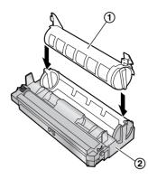
4 Firmly press down the toner cartridge to snap into position.
